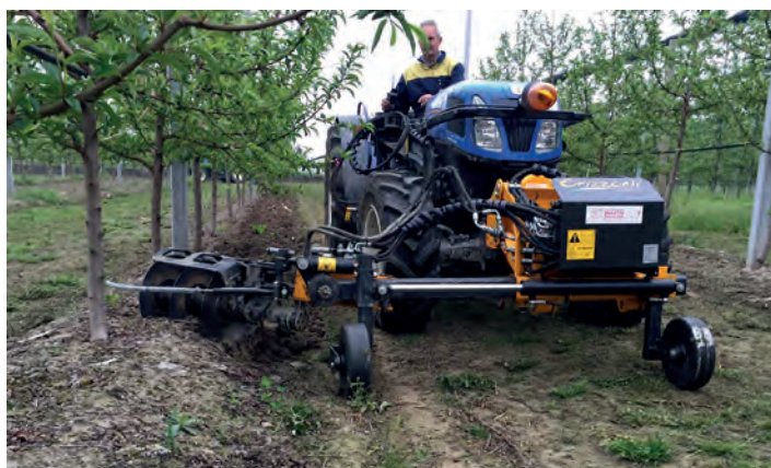
ENERGY/S con dischiera scolmatrice - ENERGY/S with motorized disc plough
